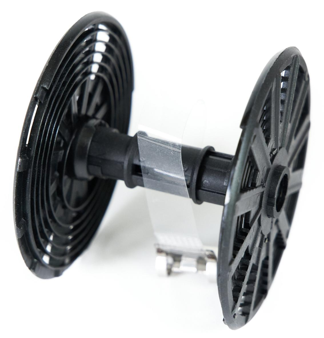
I then replaced the orange knob on the side of the Lab-Box with the optional Crank that I bought and found that the end of the crank feeds into the spool inside the tank, as you might imagine so that we can turn it later. Here I have also opened the grey lock on top of the film module on the left, ready to load my film. You can also see the reel with the film clip and film guide now in place inside the tank.
