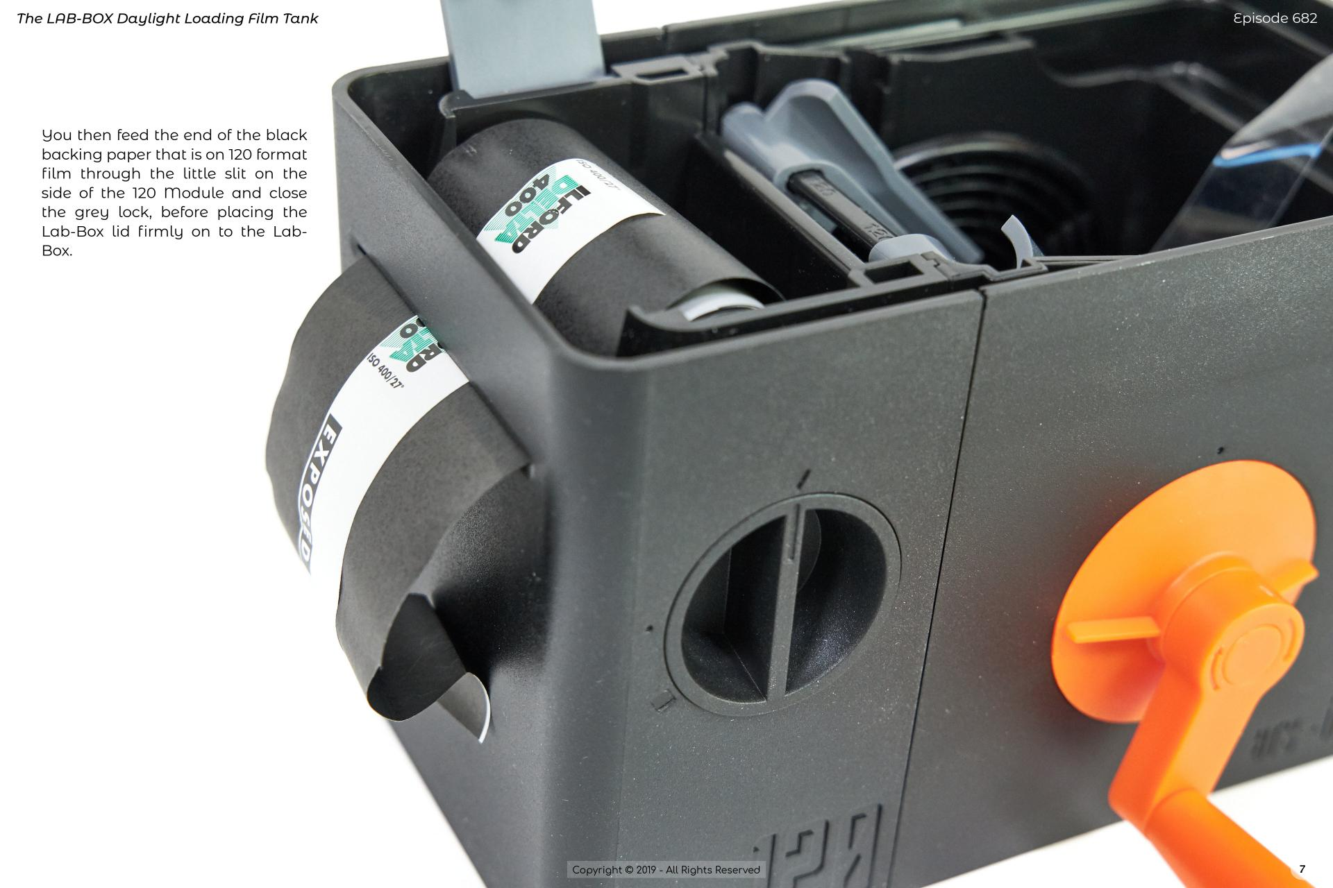
Then pull the backing paper out through the slit and this, in turn, feeds the film into the canister. You keep pulling the backing paper out until it stops. You'll see the number one on the paper showing that you've reached the start of the roll. You then close the film canister by rotating the dial to the square.
